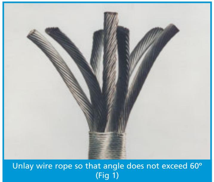
Unlay wire rope so that angle does not exceed 60° (Fig 1)
